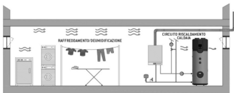
Heat pump for sanitary water with wall-mounted gas boiler
